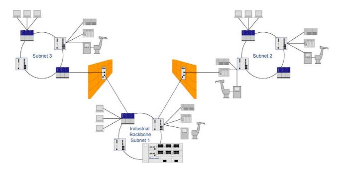
Figure Security-2: Example for secure cell separation
