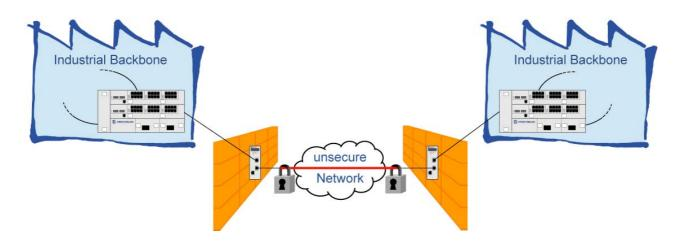
Figure Security-3: Example of a secure connection between networks
